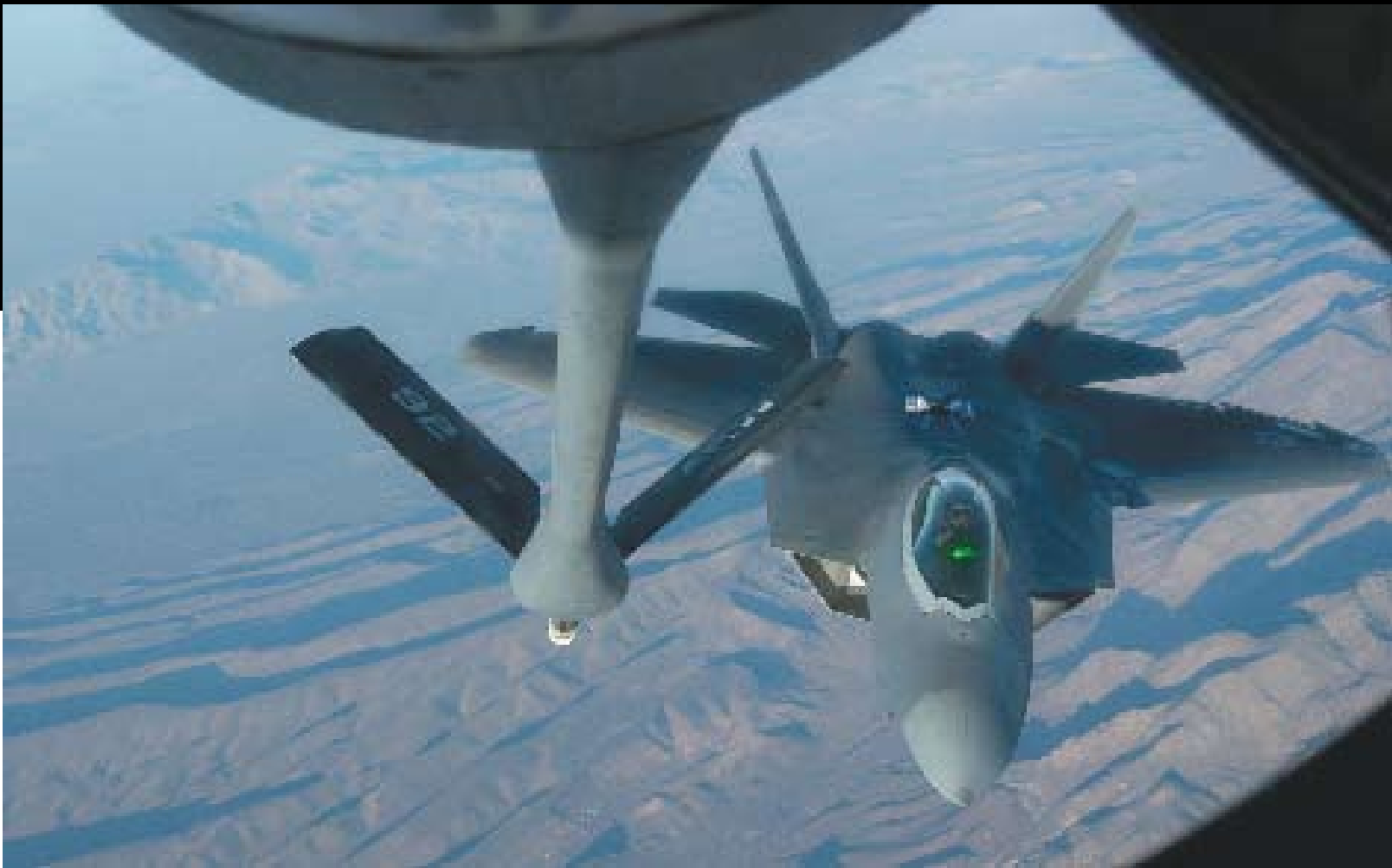
This is the view a boom operator has during a during a mid-flight refueling mission.
